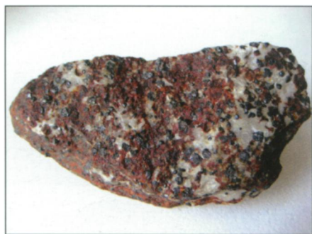
Fig. 21. Franklinite – zincite ore from a mineral collection of the Geology Department of Bryn Mawr College. The red, orange, and yellow is zincite (ZnO); the black is franklinite [(Zn,Mn 2+ ,Fe 2+ )(Fe 3+ ,Mn 4+ ) 2 O 4 ]; and the white is calcium carbonate (CaCO 3 ).
