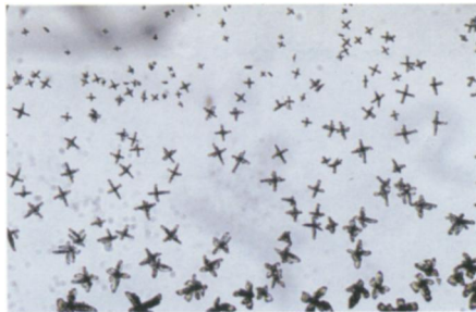
Fig. 5. Photomicrograph of microchemical test for zinc, illustrating how the crystal precipitate grows into feathery crosses that appear black in the transmitted light of the microscope (50X). The precipitate formed is a salt: [\text{ZnHg}(\text{SCN})_4] . The test confirms the presence of zinc in the orange pigment particles (zincite).
