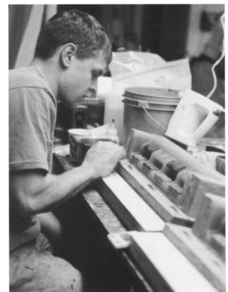
Fig. 6. J. B. and Sons craftsman delicately lays or "butters" the red and blue colored grout into the mold. Photograph by the author.
