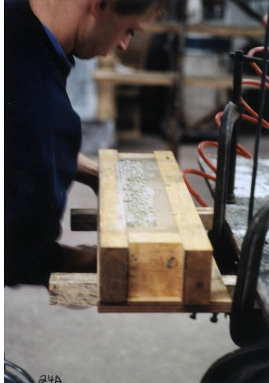
Brief vibration settles mixture into the mold, ready for reinforcement
