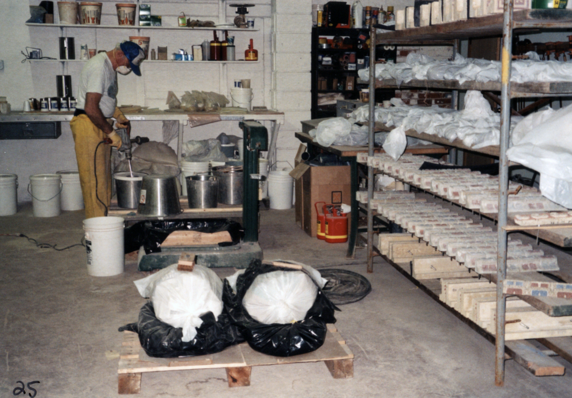
J.B. & Sons work area for measuring, mixing, and curing pre-cast elements
