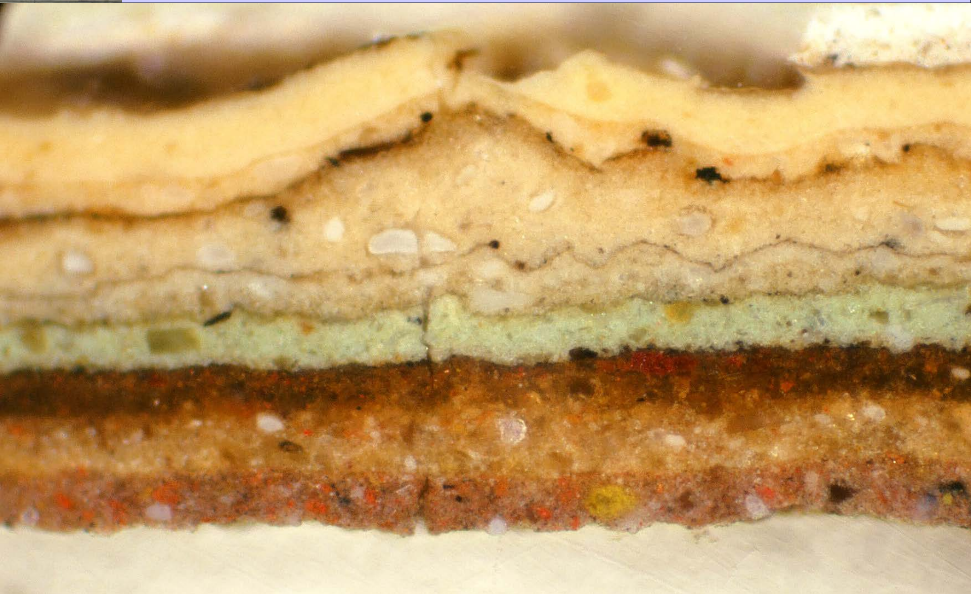
Zinc-based paint made from the crushed ore of franklinite and zincite in New Jersey
